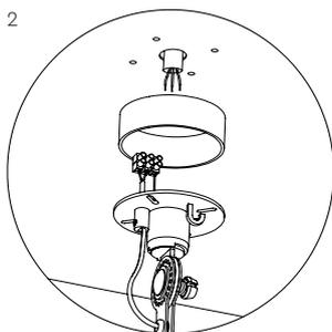
1. With terminal block to install directly on a junction box.
